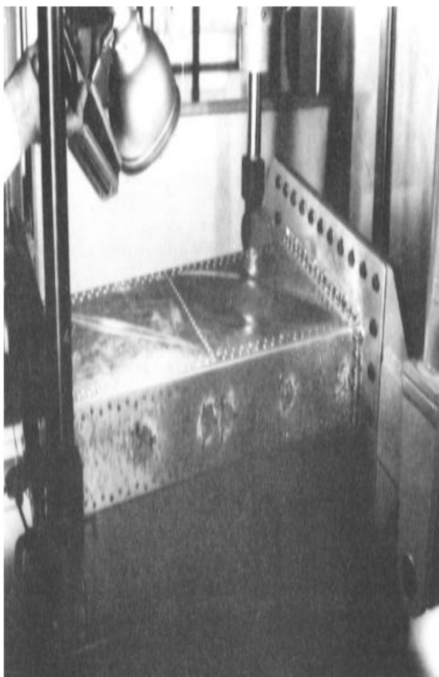
a). Torsion tests on wing boxes [13],[14].
